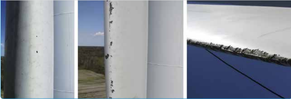
Figure 17 Evolution of Erosion of Leading Edge through Normal Wear [24]
